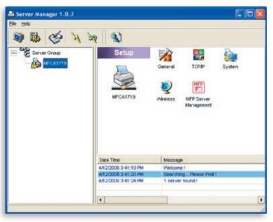
Double-click the "TCP/IP" icon and the "TCP/IP" configuration window opens. You can configure the Print Server to automatically get an IP address from a DHCP server (enabled by default), or manually specify static-IP configurations. The Print Server also has a built-in DHCP server (disabled by default).
